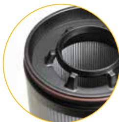
PALL UE 619 Replacement Elements Extra thick extraction ring and support ribs – prevents break-off during replacement
