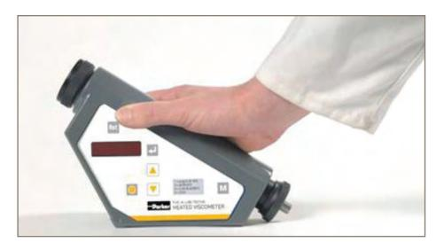
Viscosity is regarded an oils most important characteristic. It is the viscosity that shows the oil's resistance to flow and the strength of the oil film between surfaces. Viscosity can increase or decrease as a result of problems such as contamination, fuel dilution and shear thinning. Measurement of viscosity is extremely important for hydraulic oils, diesel engine oils, gears and fuel oils.
