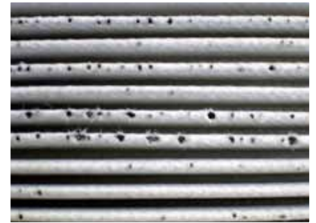
Example of holes burned in the filter media.
